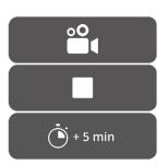
By pressing the left camera icon, a live recording will be made. By pressing the square icon, the recording will be stopped. The recording can be retrieved during surgery by selecting the "timeline" icon (see 8.4.4 timeline). After surgery, the recording can be accessed by going to the case manager (see chapter 8.4)
