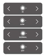
The amount of laser light can be adjusted by use of these icons. Increasing the amount of laser light results in a greater fluorescent response. By default, the laser setting is at its highest level.
