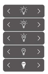
The amount of visible light can be adjusted by use of these icons. Increasing the amount of visible light has no influence on the fluorescence. Furthermore, increasing or decreasing the light is advised depending on the situation and personal preferences of the user. However, keep in mind: no visible light means no fluorescent overlay
