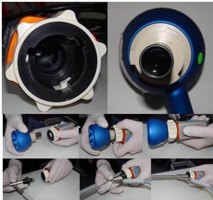
Figure 4: Connecting the ring light/Laparoscope to the camera
