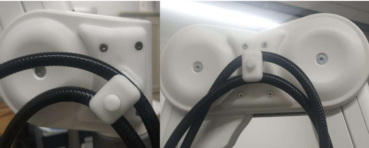
Figure 15: Cables secured in camera arm
