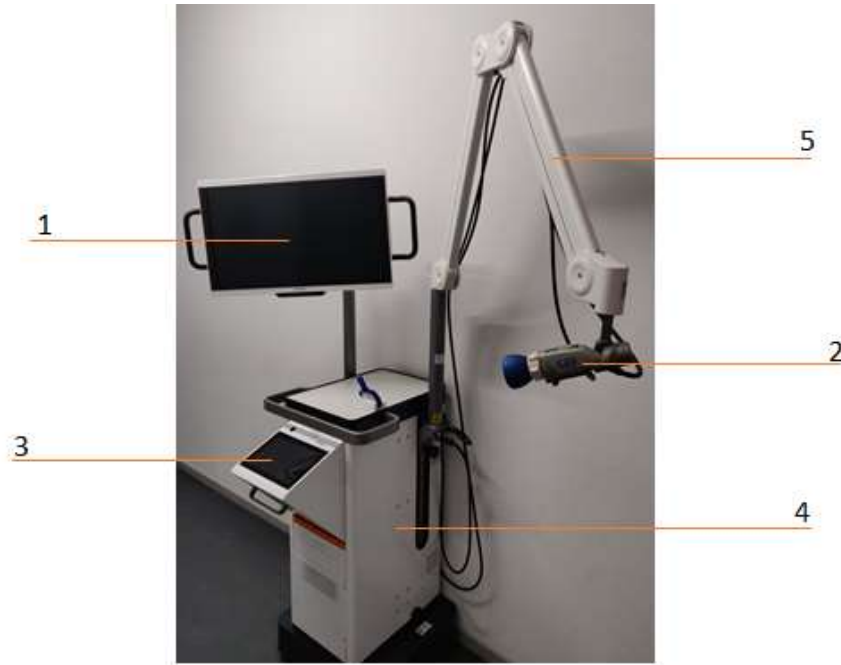
Figure 1: Overview of the QUEST SPECTRUM® 3. 1) 4K Monitor, 2) Sensitive camera, 3) Interactive touchpad, 4) Trolley, 5) Mechanical Arm
