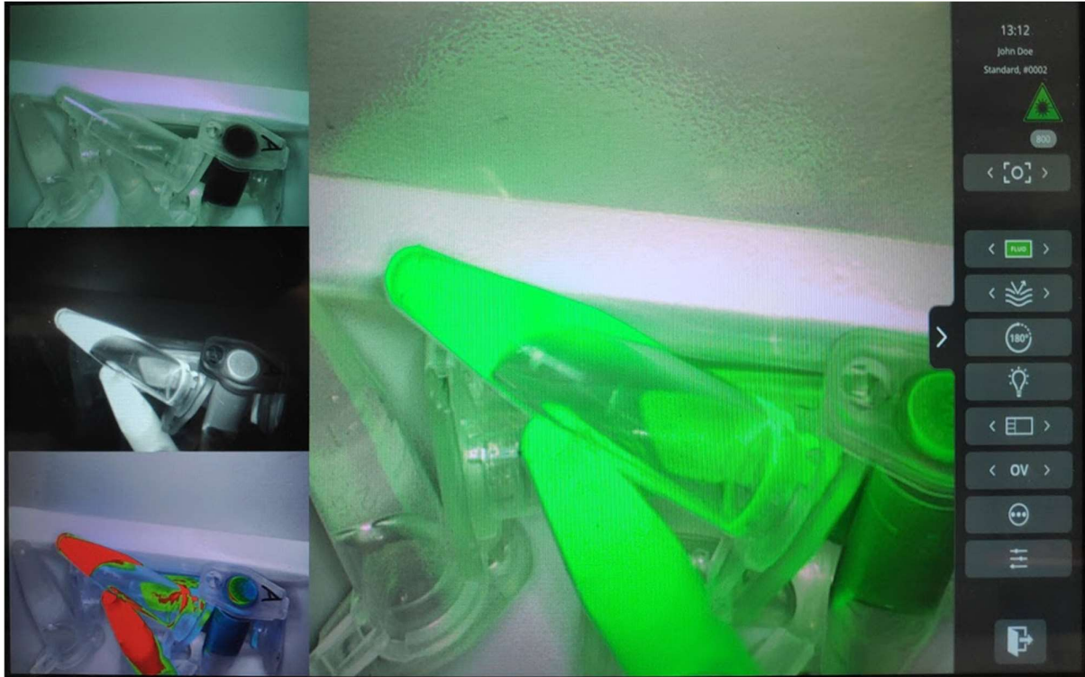
Figure 10: Surgery mode view (ICG). Main image corresponds to Overlay (OV) mode. On the left, from top to bottom: RGB, NIR, GR modes.
