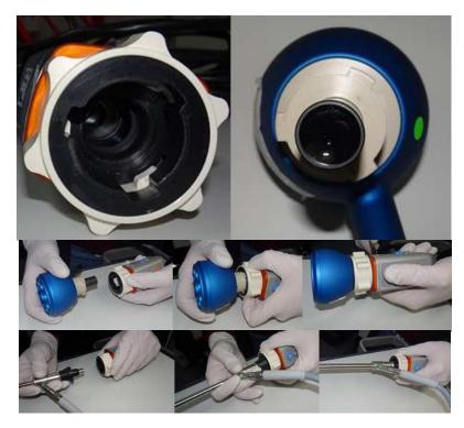
Figure 4: Connecting the ring light/Laparoscope to the camera
