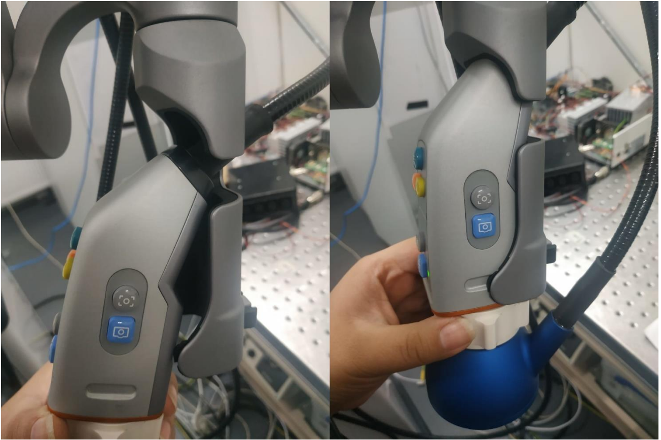
Figure 14: Camera positioned in arm gripper
