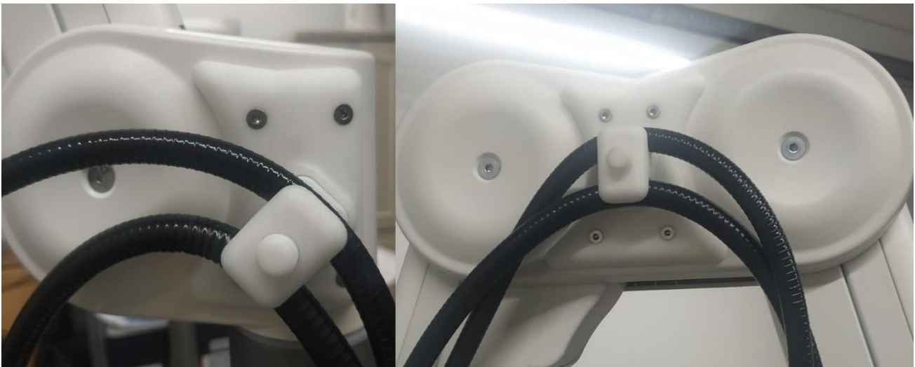
Figure 15: Cables secured in camera arm
