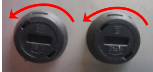
Figure 22: Replacement of the fuses
