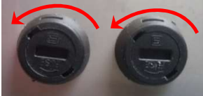
Figure 18: Replacement of the fuses
