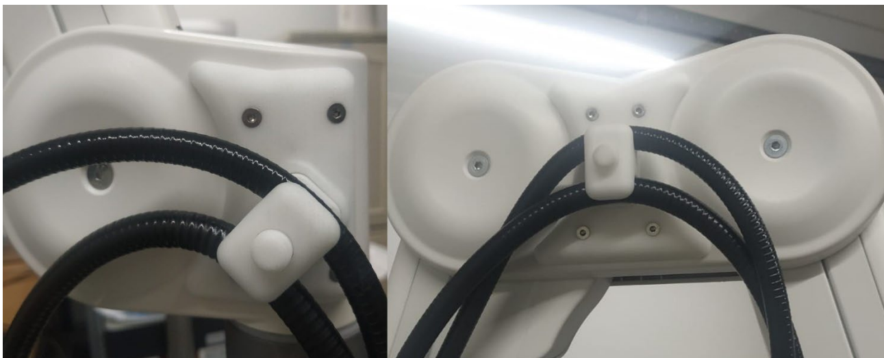
Figure 15: Cables secured in camera arm
