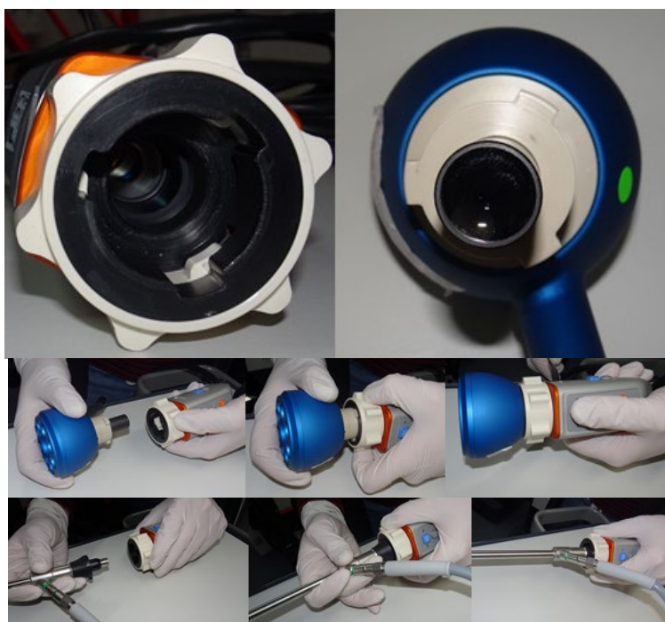
Figure 4: Connecting the ring light/Laparoscope to the camera
